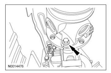
4. Remove the transmission shift linkage bolt and the gearshift lever bolt. Disconnect the shift linkage from the transmission.
