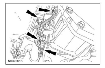
6. Disconnect the Output Shaft Speed (OSS) sensor electrical connector.
