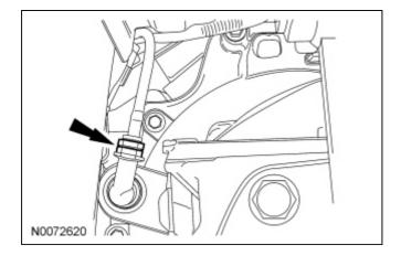
10. Loosen the exhaust coupler and disconnect the intermediate pipe from the catalytic converter. Discard the exhaust coupler.
